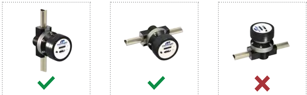
Figure 9: Meter orientation for register assembly
