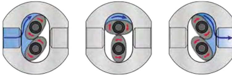
Figure 1: Macnaught Positive Displacement Flow Meter operation.
