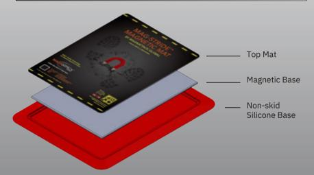
The new and improved Mag-Stride™ Magnetic Mat includes a design change to the red surround, which in previous models, was placed around the magnetic base. Now, in the new Mag-Stride™ model, the magnetic base is inserted into the red silicone surround which is specially made with a stepped retainer to hold the magnetic base in place. The top cover mat sits inside a slotted edge, securely holding the mat on the surface of the magnetic base.
