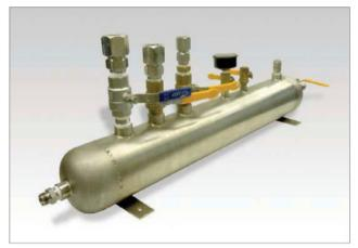
SAGE ZEROING CHAMBER One of the many data points taken during the Flow Meter's NIST calibration at Sage is at a "No Flow" (0 SCFM) condition. The Sage Zeroing Chamber is used to capture a "No Flow" (O SCFM) flow point at the actual conditions (i.e., with the same gas or gas mix and same pressure as that specified by the customer for their process)
